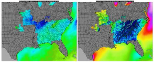
Figure 2.1: Average capacity factors for fixed latitude tilt solar (left) and 100m hub-height wind (right) over the SEEM footprint calculated from the HRRR model outputs.
