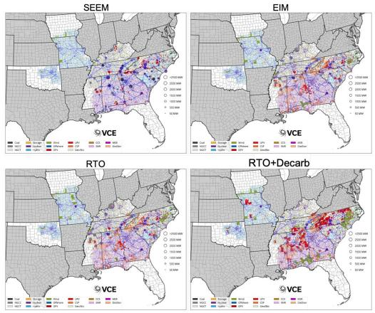
Figure 3.11: Installed generation layout in 2040 for the "SEEM" scenario (top left), "EIM" scenario (top right), "RTO" scenario (bottom left) and "RTO+Decarb" scenario (bottom right" along with transmission paths above 115 kV.
