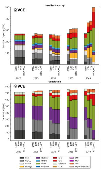
Figure 3.5: WIS:dom-P installed capacities (top) and generation (bottom) for the scenarios modeled.
