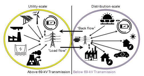
Figure 2.4: A schematic picture of the U-D interface within the WIS:dom-P modeling platform.
