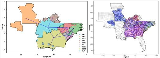
Figure 2.3: Inter-region bulk transmission and county level transmission topology for the SEEM region.
