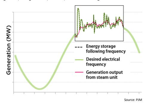
Frequency regulation refers to the need to react to short-term changes to supply and demand to maintain the frequency of the grid within its operational limits. Maintaining the frequency of the electricity on the grid is essential to ensure that it remains within the narrow range necessary to maintain system stability. System frequency that becomes too high or low can damage equipment and lead to blackouts or other grid failures.
